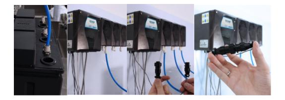
5.6 Power Up the EZChem System. Plug the pump cabinet to an available outlet. The system is now ready. If no errors are present, pumps will begin to auto prime the chemical line. If pumps do not run, the remote will indicate an error condition.
